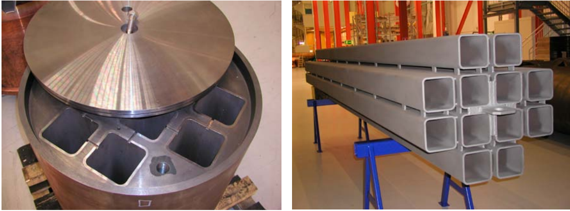
Figure 5-4. The photo on the left shows part of the machined insert with the notches between the fuel channels, and a steel lid with a hole for the valve for atmosphere replacement and a centre screw. The photo on the right shows a steel tube cassette.
