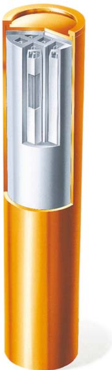
Figure 3-1. SKB's reference canister with an outer corrosion barrier of copper and an insert of nodular cast iron.
