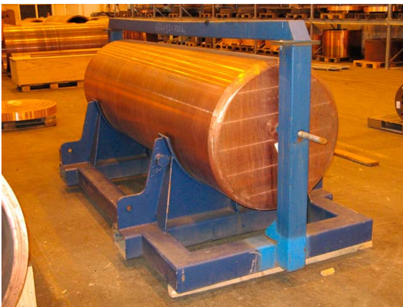
Figure 5-9. Large copper ingot weighing approximately 12 tonnes.
