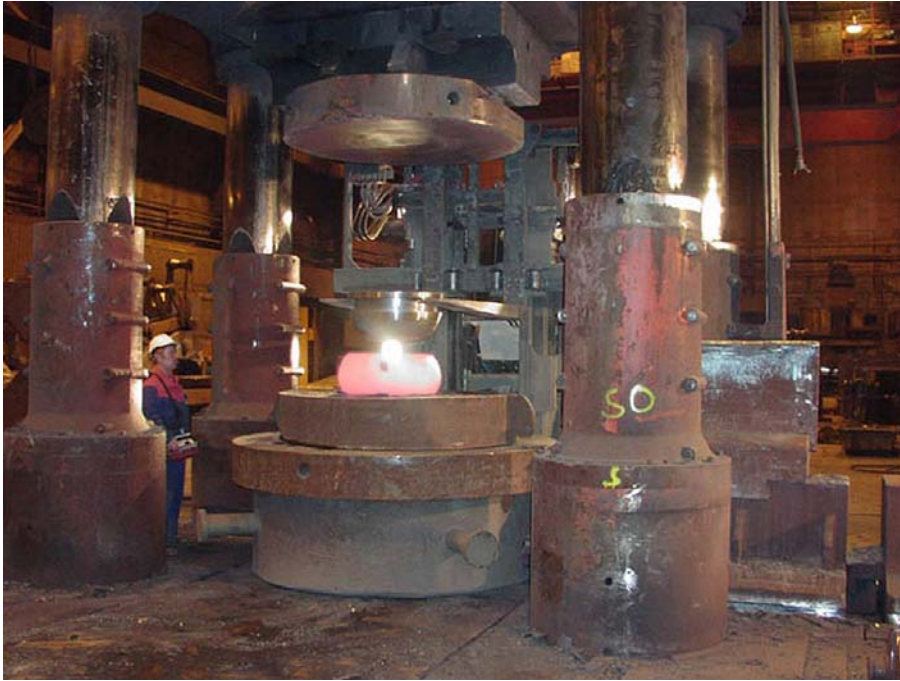
Figure 5-17. Forging of a lid blank.
