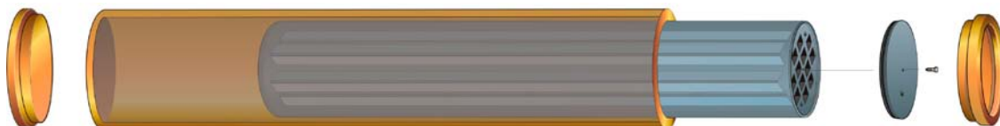
Figure 3-3. Exploded view of the reference canister and its components (from the left: copper base, copper tube, insert, steel lid for insert and copper lid).
