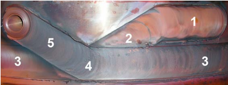
Figure 5-26. Sequences in the welding cycle: 1) acceleration sequence, 2) downward sequence, 3) joint line welding, 4) overlap sequence and 5) parking sequence.
