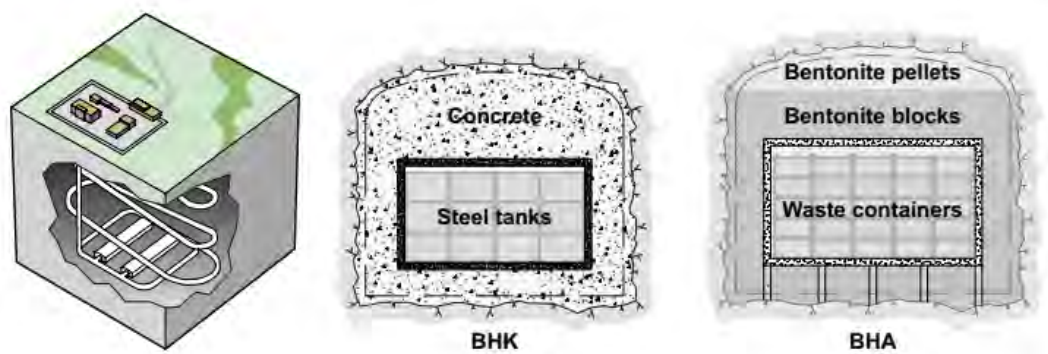
Figure 1: Preliminary facility layout and the proposed repository concept for SFL (left), with one waste vault for metallic waste from the nuclear power plants (BHK, centre) and one waste vault for waste from Studsvik Nuclear AB, Cyclife Sweden AB, and AB SVAFO (BHA, right). After SKB TR-19-01.
