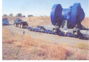
Figure 2-8 Unloading of RPV into LLW Disposal Trench
