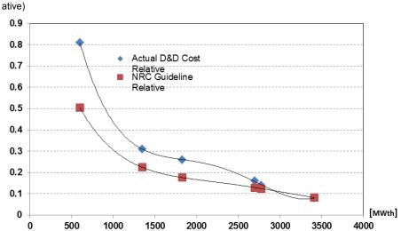
Figure 4-1 U.S. NPP D&D Cost Comparison for PWRs of Different Thermal Power (Relative)
