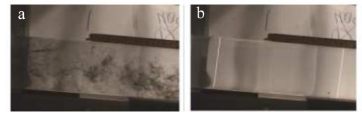
Fig. 6. A snapshot of the video recording showing the pipe and the colour transported from right to left (a); the position of the pixels used in the correlation analysis (b).
