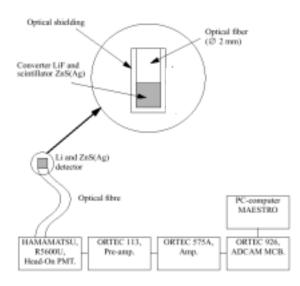
Fig. 5. The measurement system
