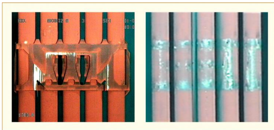
Figure 29: Appearance of Inconel spacer induced shadow corrosion on Zry-2 cladding. The photo to the right is the same assembly as shown to the left but after the spacer has been removed and the rods have been brushed to remove the loosely adherent CRUD [Châtelain et al., 2000] and [Ledergerber et al., 2006].
