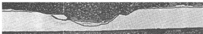
Figure 48: Cross-section of corrosion pit in cladding caused by CILC. From [Marlowe et al., 1985]
