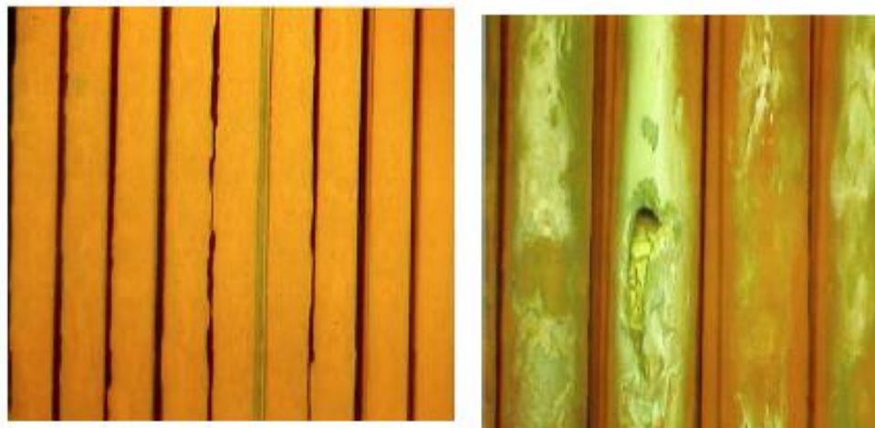
Figure 46: CRUD on BWR fuel (left) and localized corrosion failure of cladding (right) [Cheng and Yang, 2003]
