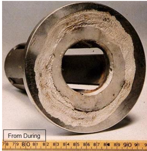
Figure 44: Stainless steel crevice corrosion [During, 1991]
