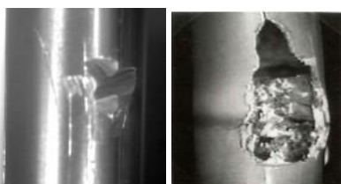
Figure 7: Leaking fuel rod (left), Damaged rod (right)
