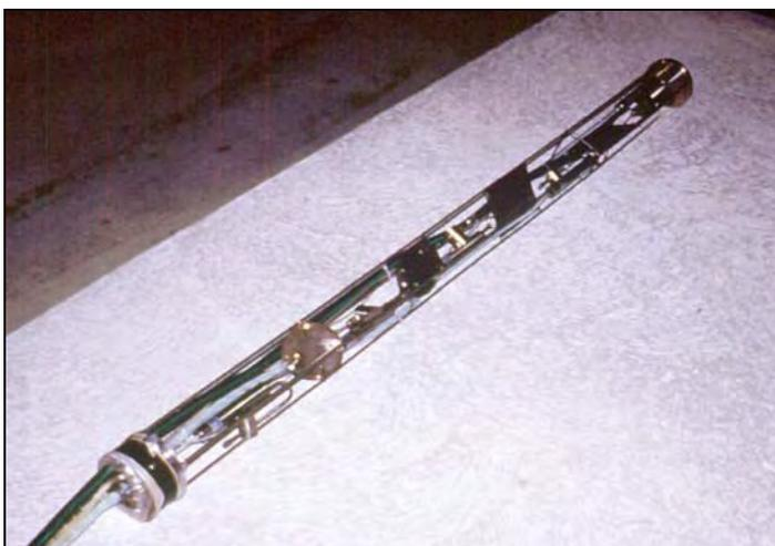
*Figure 7.2: Set of total pressure sensors for the three-dimensional measuring of stresses in boreholes in granite.*
