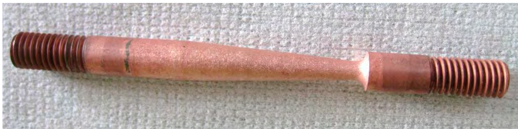
Figure 24: Photograph of specimen #6 after exposure four.
