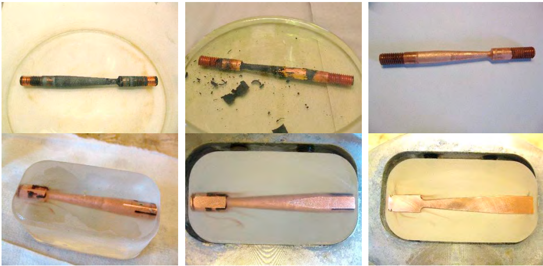
Figure 10: Cleaning in HCl (top row) and polishing (bottom row) of an exposed copper specimen.
