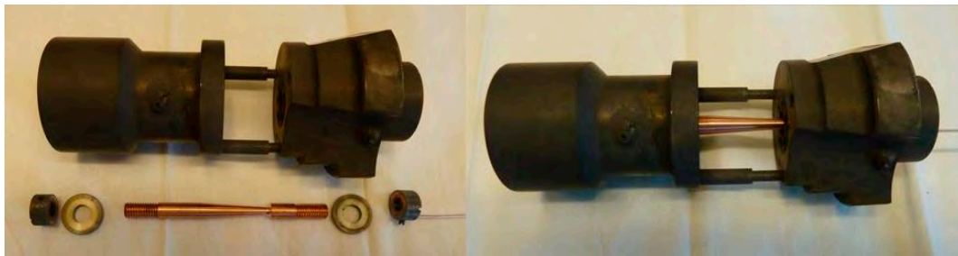
Figure 4: Photographs of a tapered specimen un-mounted (left) and mounted (right) before exposure.
