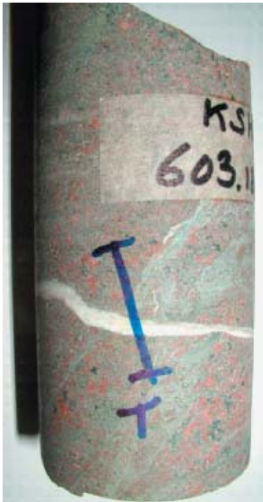
Figure 5-40. Drillcore sample KSH01A:603.11 m showing fracture sealed by prehnite (greenish) and cut by discordant calcite filling (white). Note the red staining and chloritisation of the wall rock. Blue line shows location of thin section.
