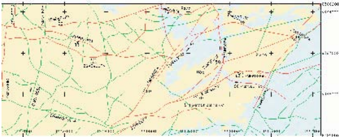
Figure 5-54. Interpreted high confidence (red) and possible (green) deformation zones in the local model domain. The top illustration (a) shows the model in perspective, (b) shows a top view corresponding to sea level (c) shows the situation at Z=-500 m.a.s.l.
