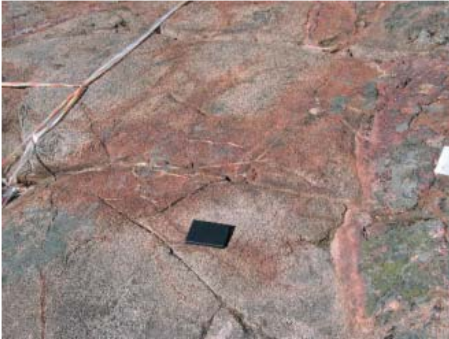
Figure 5-33. Red staining along sealed fractures in quartz monzodiorite, Simpevarp peninsula. The mineral filling is presumed to be dominated by prehnite. Outcrop ASM000206 where detailed fracture mapping has been carried out (cf. Figure 5-17 and Figure 5-30). The size of the black note book is 16.5×13 cm.
