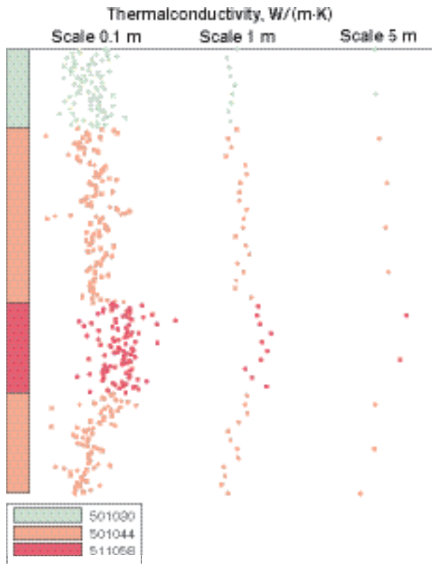
Figure 7-8. Conceptual illustration of effects of applying the principle for upscaling of thermal conductivity, as given in Figure 7-7, where mean values, standard deviations, and lower and upper confidence intervals for the domains are calculated for different scales.
