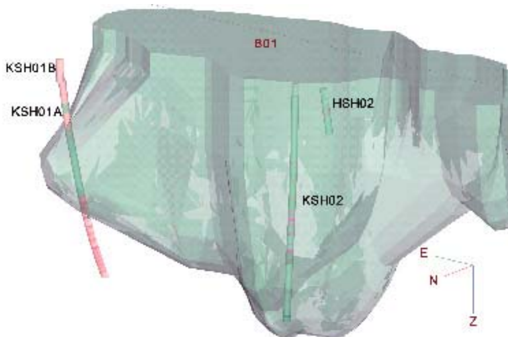
Figure 11-3. Rock domain RSMB01 that is dominated by fine-grained dioritoid. Simpevarp peninsula. View from the northwest.
