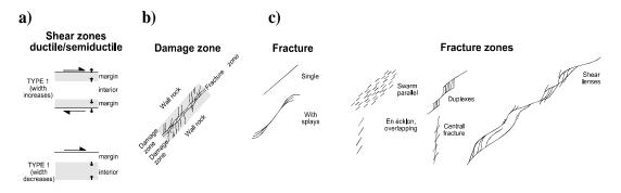
Figure 31. Geometry of deformation zones: a. deformation along shear zones (Means 1984 and 1995), b. wall rock damage zone at a shear zone or fracture zone, and c. deformation along fractures and fracture zones.
