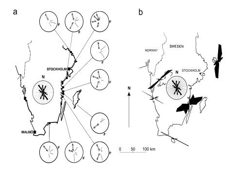
Figure 7. Orientation of tectonic structures: a. faults mapped along the Swedish East Coast (SKBF/KBS, 1983) and F is orientation of the foliation, and b. clastic Cambro-Ordovician dykes (Bergman, 1982). The rose diagram in the centre of figures gives the orientation of kursu-valleys.
