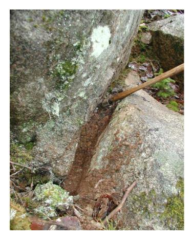
Figure 24. In situ blocks with rounded corners and a fracture fill composed of grus weathering product (brownish in colour, see section 4.1).
