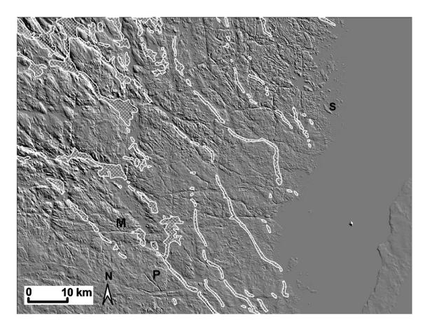
Figure 5. Digital terrain model, relief map (LMV elevation data base, 50 by 50 m grid), illuminated from NE, size of the area is 100 by 75 km. Distribution of glaciofluvial sediments, preferentially eskers, are displayed. Location of over-deepened valleys mention in text: Moredalen (M), Pukedalen (P), and a submarine canyon, Strupdjupe (S). Permission to publish by the National Land Survey of Sweden (I 2007/1092).
