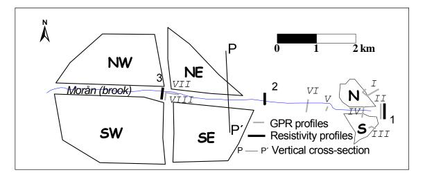
Figure 16. Simplified map showing the location of : a. four rock blocks (NW, NE, SE and SW) see text and Table 1, b. northern part and southern part of the delta (N and S) see text, Figure 17 and Table 2, c. GPR profiles (grey lines, I to VIII), see text and Figure 18, d. resistivity surveys (heavy lines, 1 to 3), see text and Figure 19, and e. vertical cross-section P to P', see text and Figure 10.
