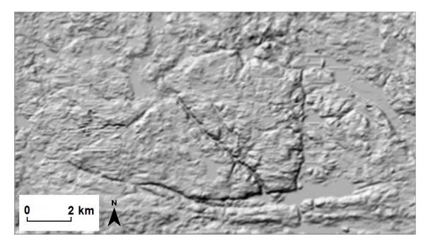
Figure 21. Digital terrain model showing the Pukedalen valley, relief map, covering an area of 18 by 10 km (LMV elevation data base, 50 by 50 m grid), illuminated from NNW. Location of the area is given in Figure 4. Permission to publish by the National Land Survey of Sweden (I 2007/1092).
