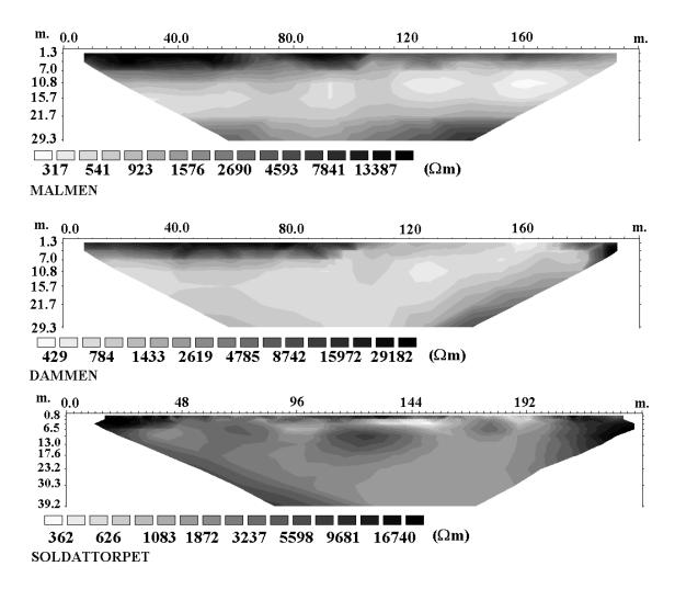
Figure 19. Resistivity inversion model sections, profiles 1 (Malmen), 2 (Dammen) and 3 (Soldattorpet). Location of the profiles is given in Figure 16. All profiles are measured from north to south.
