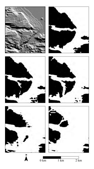
Figure 17. Illumination of the difference in elevation of the northern and southern part of the delta just east of the Moredalen valley. Altitudes above 92, 93, 95, 97 and 99 m a.s.l. are shown. Permission to publish by the National Land Survey of Sweden (I 2007/1092).
