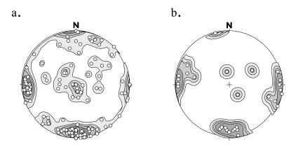
Figure 15. Orientation (poles) of fractures: a. Fractures mapped on the northern side of the Moredalen valley (n=150), and b. fractures mapped on the southern side (n=33). Schmidt projection, lower hemisphere, contours; 1, 2, 3, and 5 %.
