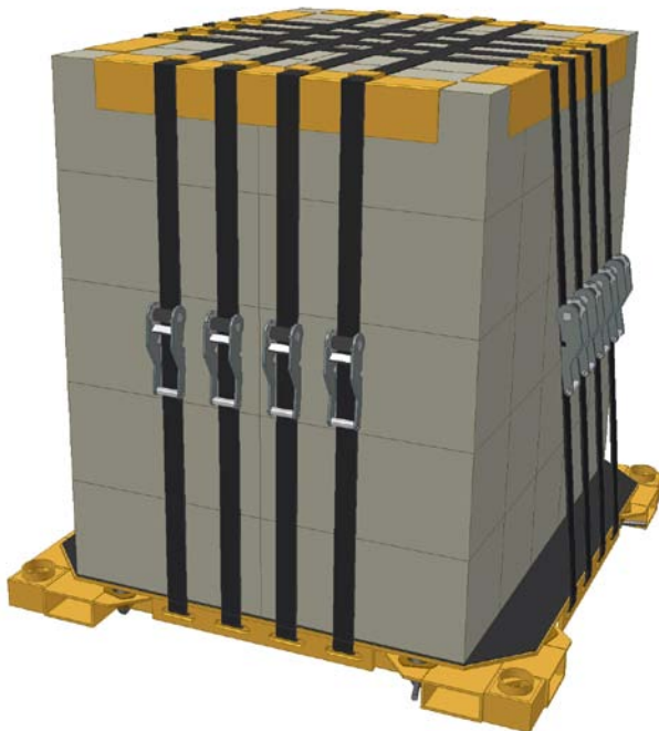
Figure 5-10. Backfill blocks placed on a special designed pallet.
