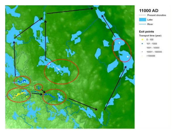
**Figure 7-7.** Illustration of the work to identify biosphere objects. The discharge points are displayed on the landscape development model (here shown without sediment dynamics, lake infilling and vegetation type/land use) for a specific time step (11,000 AD). The discharge clusters are encircled in red where the biosphere objects were identified and the black arrows indicate the surface water flow paths. Figure from /Lindborg 2010/.
