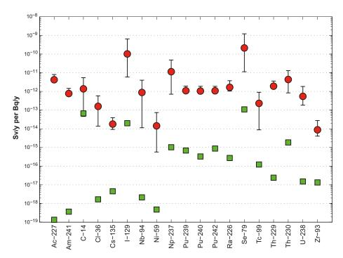
**Figure 10-4.** Mean (red circles), minimum and maximum LDF for a selection of radionuclides across biosphere objects (excluding object 105). The LDF values for object 105, which is submerged during the whole interglacial, are shown separately (green squares). Figure from /Avila et al. 2010/.
