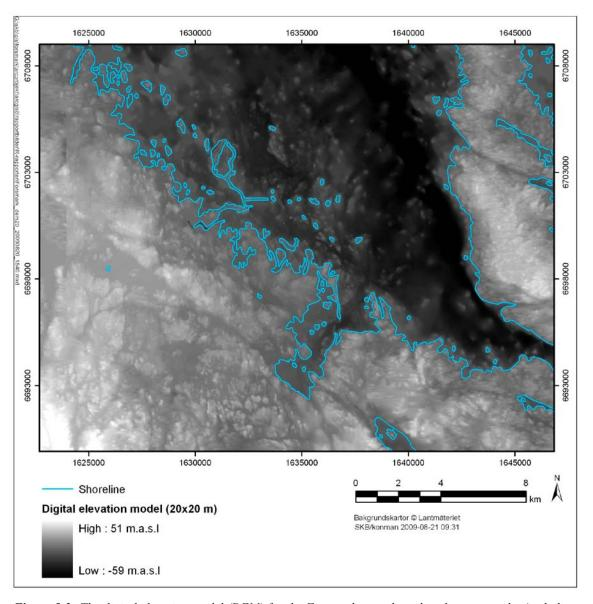
**Figure 5-3.** The digital elevation model (DEM) for the Forsmark area describes the topography (including the present-day bathymetry). The current shoreline is illustrated by a light blue line. Figure modified from /Strömgren and Brydsten 2008/.
