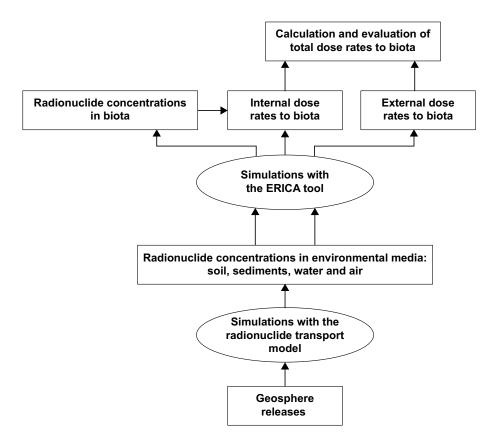
Figure 11-1. Assessment of the consequences of radionuclide releases for non-human biota. The assessent starts by calculating radionuclide concentrations in environmental medias. These concentrations are then used as input data to the ERICA tool, and the resulting dose rates are compared to a screening dose rate. Each step in the calculation procedure are explained in Sections 11.2.1 to 11.2.8 below, and details are provided in /Torudd 2010/. Figure from /Torudd 2010/.
