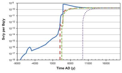
**Figure 12-1.** Effect of start and duration of release on LDF for I-129. Annual dose per unit release is shown as a function of release start and time. In the simulations 1Bq/y was released to biosphere object 121\_03 at the beginning of the interglacial period (blue line, SR-Site LDF), at the start and end of lake isolation (red and green lines respectively) or at the end of the interglacial period (purple line). Figure from /Avila et al. 2010/.
