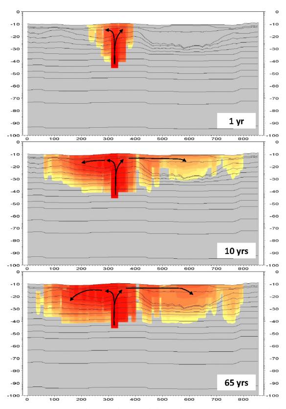
**Figure 7-6.** Concentrations after 1, 10 and 65 years of advection-dispersion simulation of transport from a single canister position. The source in MIKE SHE is at –40 m.a.s.l. along a flow path identified by particle tracking in the ConnectFlow model. Red colour indicates high and yellow low concentration. Figure from /Bosson et al. 2010/.
