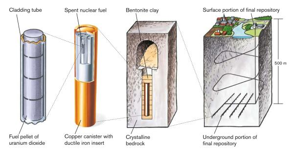
Figure 3-1. The KBS-3 concept for storage of spent nuclear fuel.
