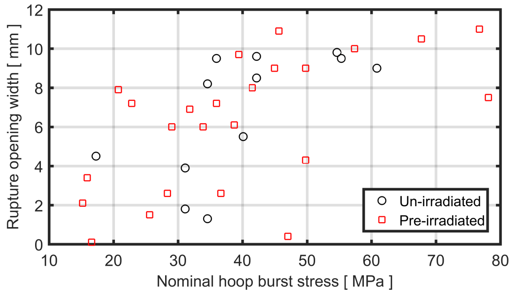
Figure A.14: Measured rupture opening width, w_b , versus nominal hoop burst stress, \sigma_b , for the FR2 test rods.
