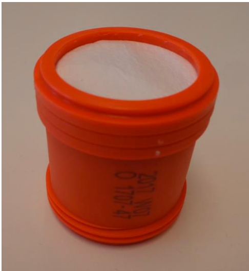
Figure 3-6. Aerosol filter used for activity monitoring in the main stacks at B1 and B2.
