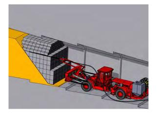
Figure 2.5 Illustration of backfill pellet emplacement. The pellets are shown in yellow (from SKB 2010b, TR-10-16).
