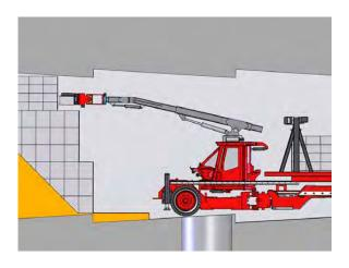
Figure 2.4 Illustration of backfill block emplacement (from SKB 2010b, TR-10-16).
