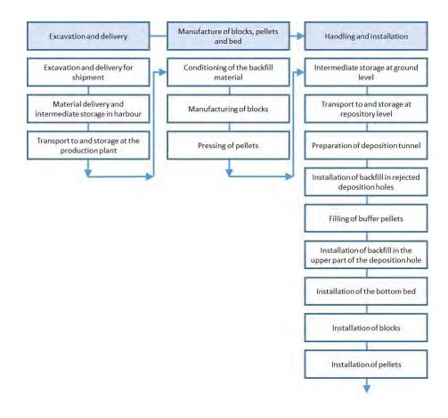
Figure 2.3 SKB's flowchart for backfill production (after SKB 2010b, TR-10-16).
