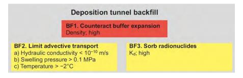
Figure 2.1 SKB's backfill safety functions (from SKB 2010a, TR-11-01)
