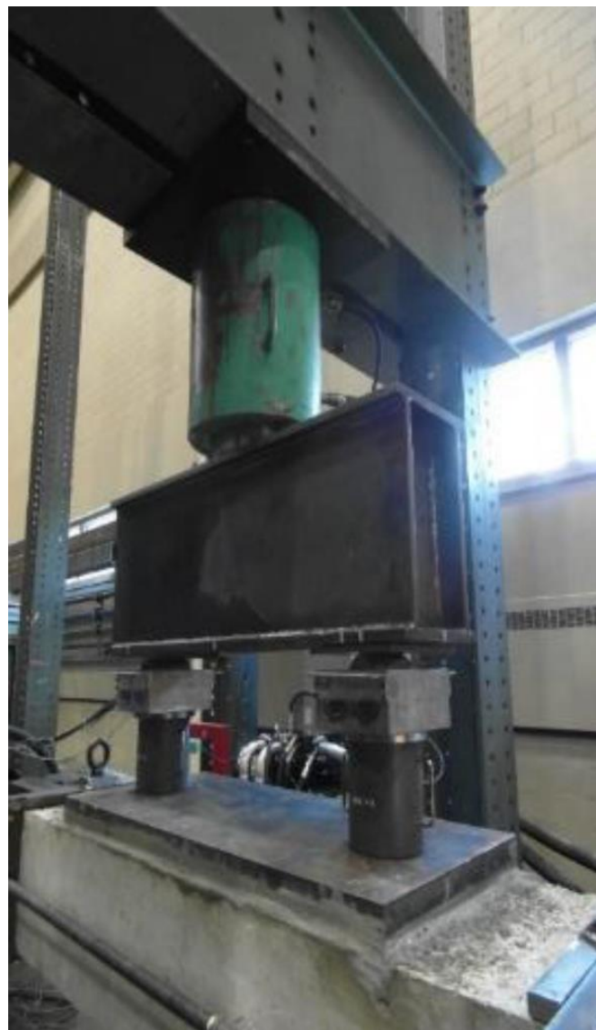
Figure 2-8 Set-up for axial loading [15].
