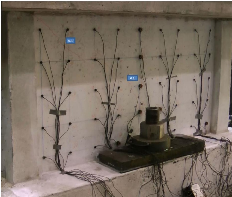
Figure 2-35 First crack at a load of 784 kN and a displacement of 1 mm of ASR A1 shear wall [15].
