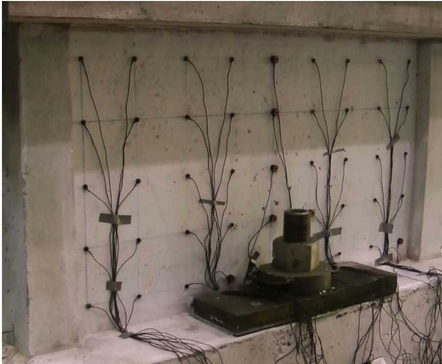
Figure 2-32 ASR A1 shear wall [15].
