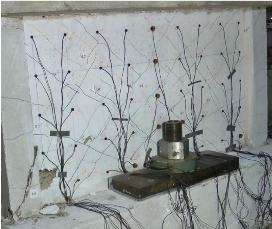
Figure 2-39 Failure (cracks width not measured) of ASR A1 [15].
