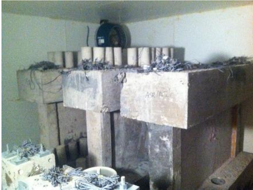
Figure 2-3 ASR test specimens in the acceleration chamber with increased temperature and humidity [14].
