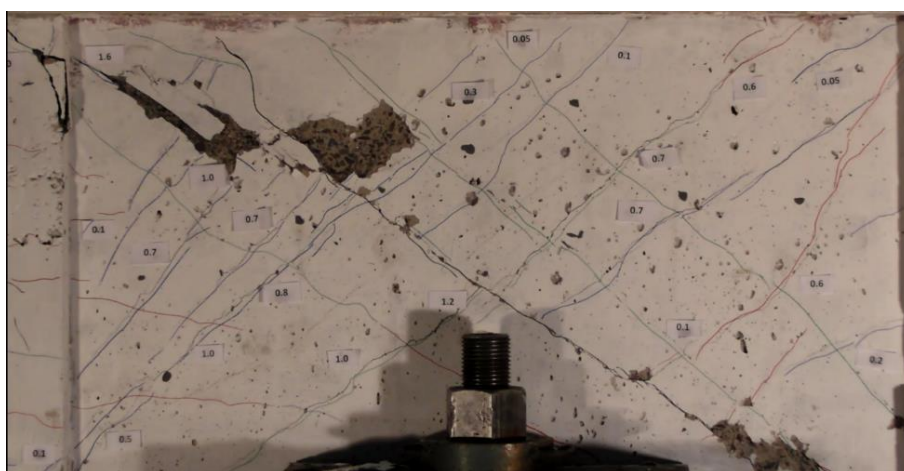
Figure 2-48 Failure (cracks width not measured) of ASR B1 [15].
