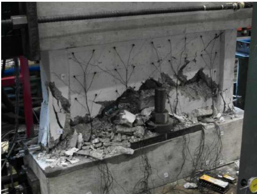
Figure 2-22 Picture of wall specimen REG A (control specimen with normal concrete) at failure [7].
