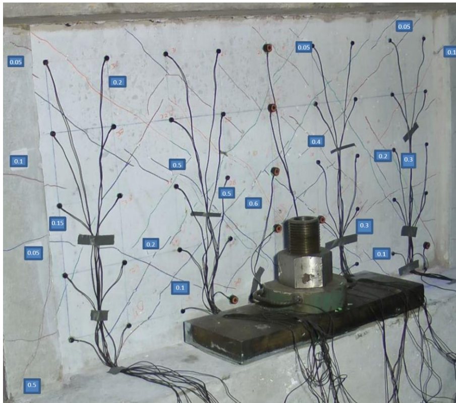
Figure 2-37 Peak load 1354 kN and a displacement of 5.2 mm of ASR A1 shear wall [15].
