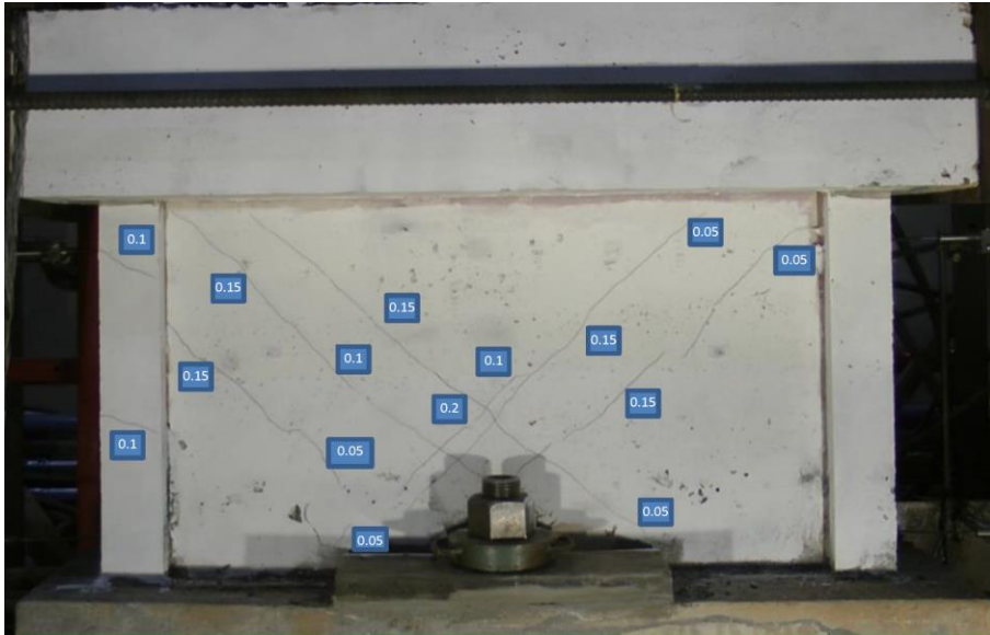
Figure 2-27 First rebar in boundary element yields at a load of 915 kN and a displacement of 2 mm Reg B shear wall [15].
