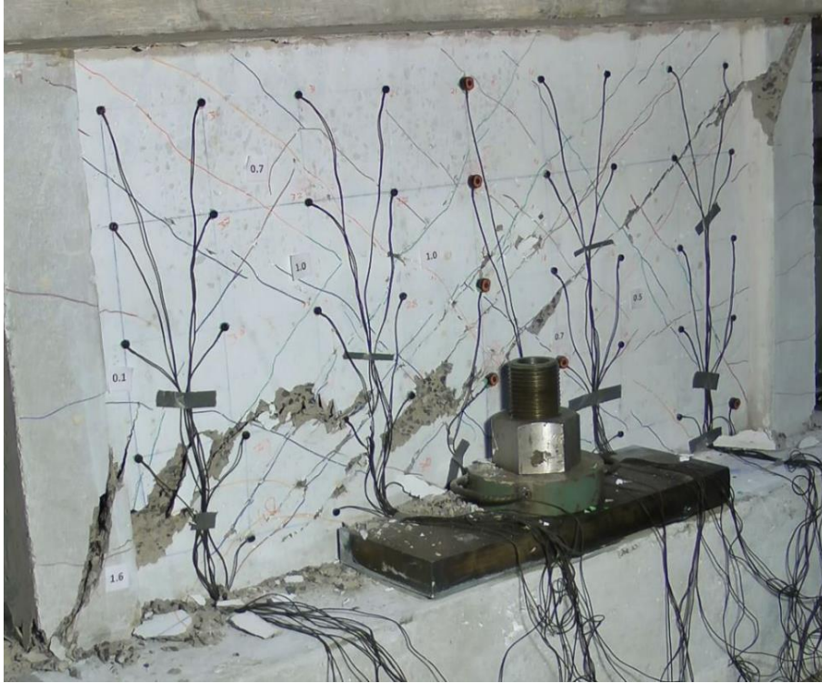
Figure 2-40 Failure (cracks width not measured) of ASR A1 [15].
