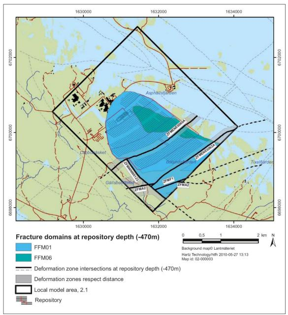
Fig. 11. Reference design layout for the repository at Forsmark, showing respect distances and the deformation zones requiring the respect distances. Fig. 5-6 from SKB TR-11-01.
