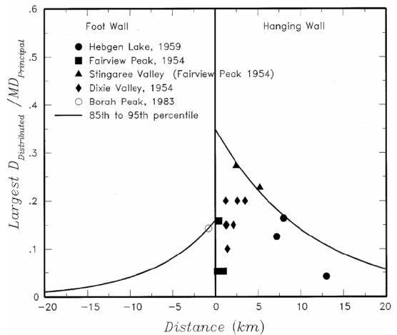
Fig. 12. Data for larger displacements on distributed ruptures divided by the maximum displacement on the principal rupture, for a set of five normal fault surface-ruptures in the USA. The curves represent a high percentile (e.g., 85th to 95th) of the distribution for D<sub>distributed</sub>/MD<sub>principal</sub>. The data were compiled by C. dePolo for the Yucca Mountain PSHA (Stepp et al., 2001).
