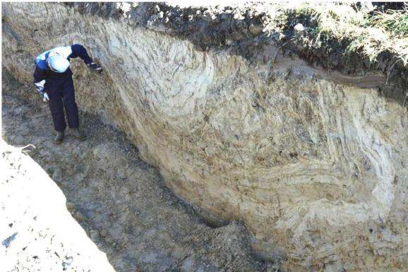
Fig. 10. Photograph of strongly contorted and folded clay at Marka (E6), about 25 km south of Forsmark. From Lagerbäck et al., 2004, Figure 5-8. The original caption describes this exposure as "Abruptly cut folds in glacial silt at Marka (E6) indicate substantional erosion of a formerly thicker sequence."
