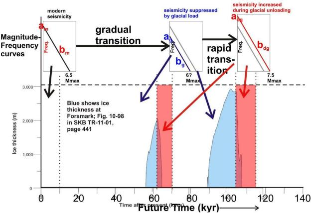
Fig. 6. Conceptual view of seismicity through the next 100,000-year glacial cycle. The lower half of the diagram shows the thickness of glacial ice at the Forsmark site (in blue) during the growth of the next ice cap. The red box marks the 10 kyr period of rapid deglaciation at the Forsmark site, when crustal rebound 12
