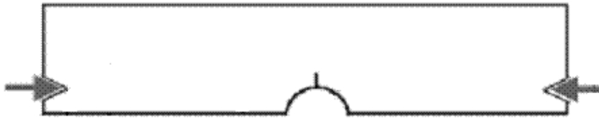
Figure 3.1. In-plane compression of the notched test specimen.
